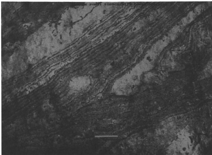
*Figure 18. Laser scanning confocal microscope image of the same structure as shown in Figure 15. In this case the sample was not frozen but shows the same ordering of the clays.*
