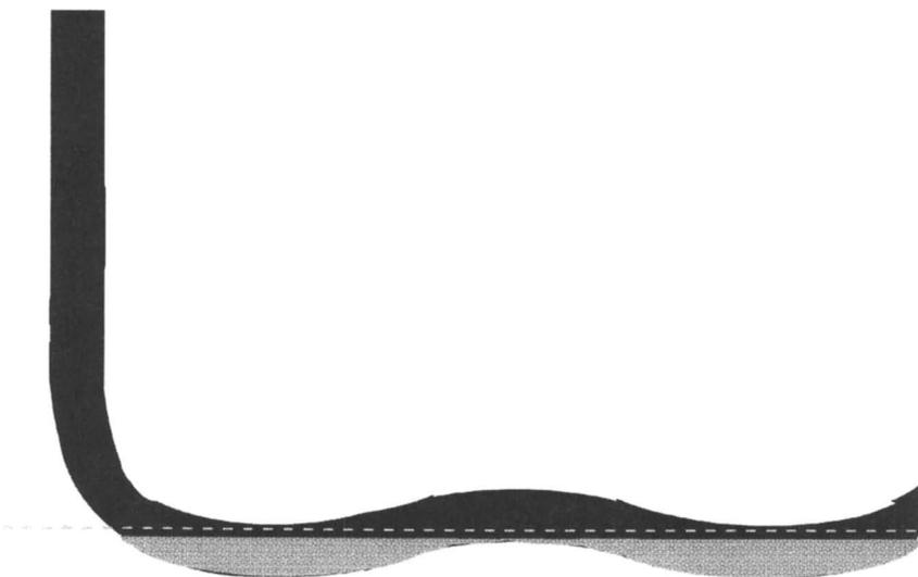
*Figure 2. Sand accumulation in horizontal wells. Complete plugging is possible when sinusoidal amplitude  $\geq$  wellbore diameter. There is also the potential for development of longitudinal annular flow. (Reproduced with permission from reference 118. Copyright 1993 Nowasco Well Service Ltd.)*
